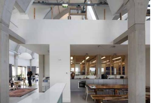
↑ Clerestory glazing faces north to reduce overheating, with curtains to screen off ground-floor windows
